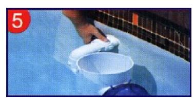
**5.** Attach the combination of union (stub, o-ring, connecting ring nut), elbow, clip-on bag, and body to your pool return jet by screwing on the connecting ring nut. Align the PoolSkim so that it is correctly positioned. The body of the unit should be approximately 2-2.5 inches (5-6 cm) below the water level. Next, tighten the screws and the connecting ring nut.
